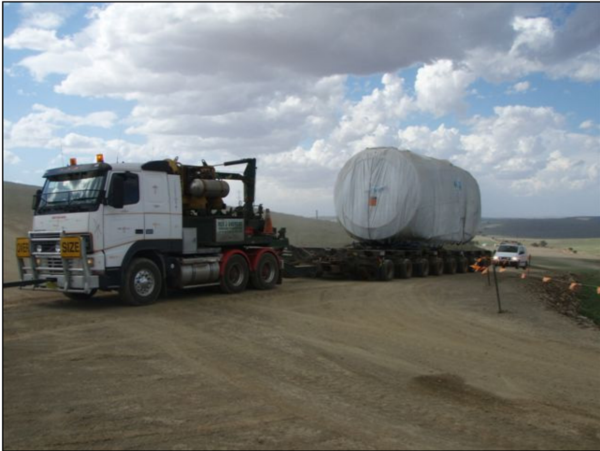
Figure 17.0 Transportation of a turbine nacelle with pilot vehicle at rear
