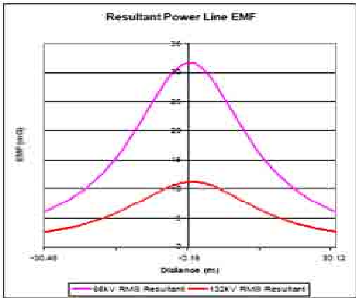
Figure 19.8 Typical 66,000 & 132,000 Volt Line EMF Profile (Vemtec 2008)
